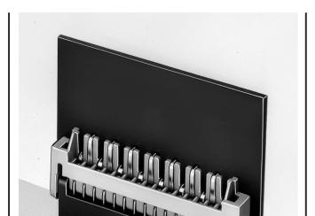
Hinge type board to board connectors which allow mated PCB's to move 90° in respect to one another while electricity is turned on. The hinge compensates for slight misalignments between circuit boards to assure a secure connection even if the boards are laterally out of line.
